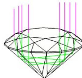
*GemRay's* black circle is an approximation to a disembodied head above the gemstone. *GemRay's* head shadow half-angle is by default 10°. How significant is this? Well, how big is your head? My head is about 10 inches (25 cm) from chin to the top of my head, so let's say it has a radius of 5 inches (12.5 cm). To what viewing distance does this correspond?
