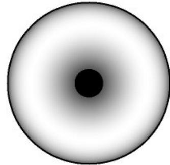
The ISO, COS, and SC2 light models don't allow any light from behind the stone, as if the room is carpeted with black carpet. In these three models, the stone is surrounded with a bezel that prevents any light from hitting the back of the gemstone. (What *GemRay* considers to be the "back" depends on how the stone is rotated.)
