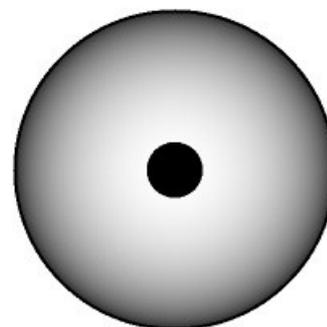
New in *GemRay for Windows* is the SC2 light model. SC2 stands for sine times cosine times two. It is white at a 45° elevation and black directly overhead and black on the horizon. It is sort of a fuzzy doughnut of light.
